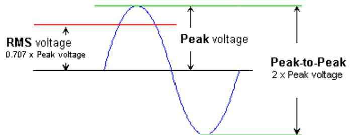
The easiest voltage amplitude parameter to measure when viewing a pure sine wave signal on an oscilloscope is its peak-to-peak voltage. The relationship between the **peak-to-peak** voltage and the **peak** voltage amplitude of a symmetrical waveform is 2:1.
